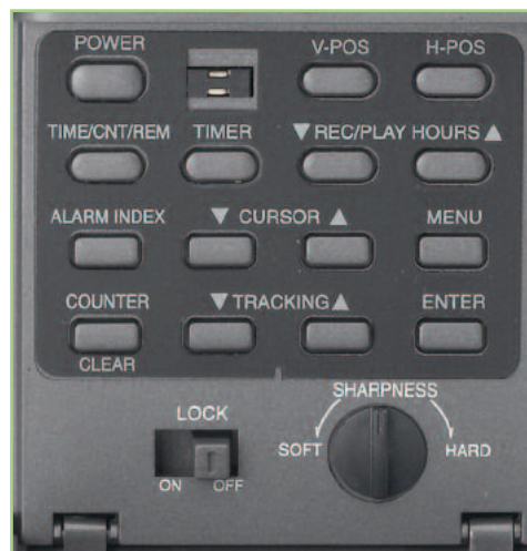
CTR-030NC-2 control panel
